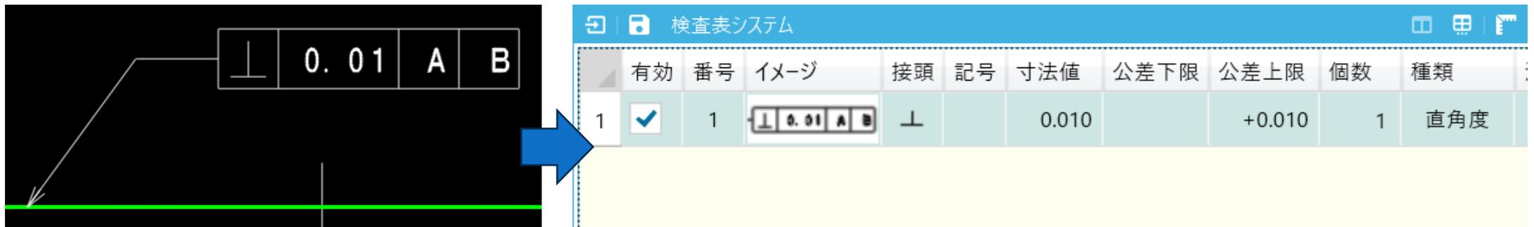
The diagram illustrates the process of registering a geometric tolerance symbol into a system. On the left, a technical drawing shows a perpendicularity symbol (⊥) with a tolerance value of 0.01 and feature letters A and B. A blue arrow points from this symbol to a table in a software interface titled "検査表システム" (Inspection Table System). The table contains the following data:
